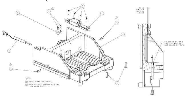
Figure 41: PR70 Base Frame Assembly (LC0109)
